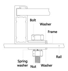
Figure 6. Bolt installation methods
