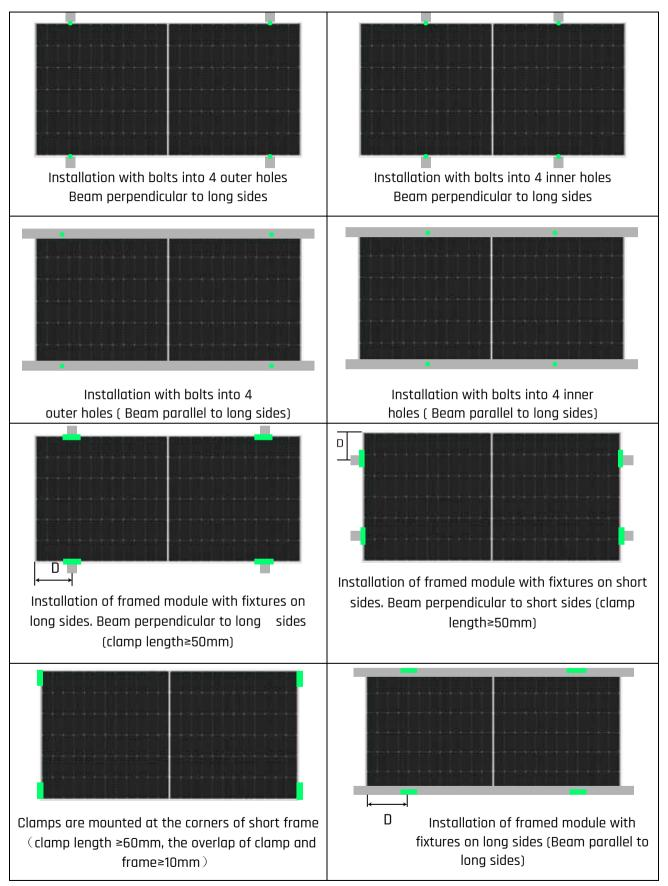
Figure 6. Specific installation of clamps
