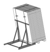
Gently push the assembly so that it leans against the support frame and remove the vertical steel strip
