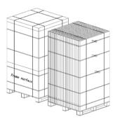
Use scissors to remove the three transverse steel strips from the upper part of the assembly
