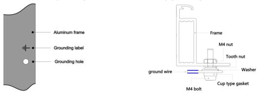
Figure 1. Ground hole and its identification
