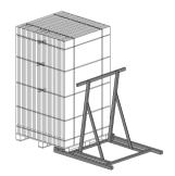
Place a support bracket on either of the recline surfaces of the assembly and remove the three transverse steel strips from the upper part of the assembly with a cutter
