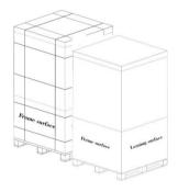
Remove the plastic wrap and wrapping film for the modules to be removed, and remove the cover and packing case
