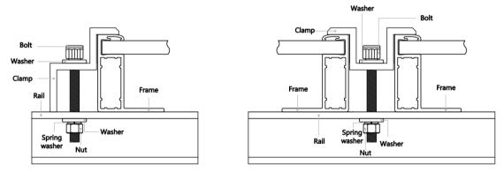
Figure 7. Specific installation of clamps
