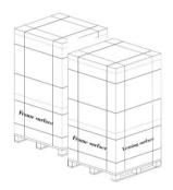
Unpacking the reclining surface needs to be close to a solid wall or another pallet of intact components of the same size
